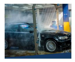
**Full-Service Most Often:** Used a full-service car wash that pulls the vehicle on a conveyor while the equipment cleans the vehicle on the outside and the interior is cleaned manually
